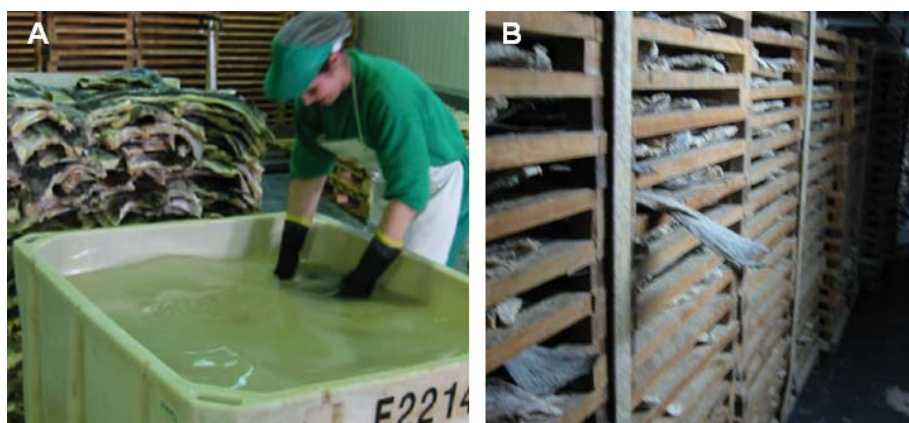
Figure 6.3.3: Washing the green fish (A) before the drying tunnel (B; photos: Svanhild E. Haugnes).
