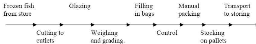
The other production line one is used for processing of fish products in boxes, such as fillets of cod, saithe etc and functions in the following way:
