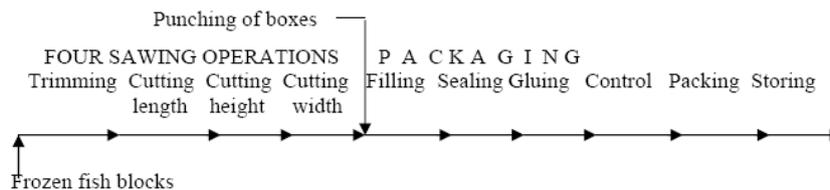
In the three cutting operations the fish blocks can get various shapes owing to the actual adjusting of the saws. As a complement to the flowchart it can be mentioned that there are also three manual packaging lines and one line for bulk packaging. It is important that the process throughput time is minimised to secure the quality of the products. In some cases it is limited to half an hour, while in some operations the process takes 2 hours.
